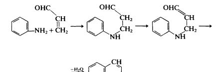
A mixture of aniline and  $C_8$ — $C_{15}$ -alkylated anilines (45%  $C_{12}$ , 15%  $C_{11}$  and 12%  $C_{13}$ ) in an acid medium is heated up to a temperature of 140°C for 12 hr, after which acetone is added. The final product is an oil containing 58% 6-dodecyl-1,2-dihydro-2,2,4-trimethylquinoline, 6% dodecyl aniline and oligomer 1,2-dihydro 2,2,4-trimethylquinoline.<sup>69,70</sup>
