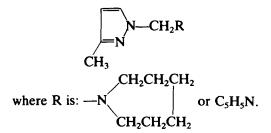
The ozone resistance of rubber mixtures based on natural rubber with ozonin-16(pyperidinomethyl-35-methyl pyrazole) and ozonin-51 (hexamethyleneimino-3,5-methyl pyrazole) exceeds 1.5 to 2 times that of mixtures containing 2246 (2,2'-methylene-bis-4-methyl-6-tert butylphenol) and is close to that reached by tributylcarbamide. A mixture of ozonin-16 or ozonin-51 with 2246 in a ratio of 1:1 displays the highest activity.<sup>79</sup>
